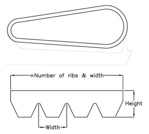
$\begin{aligned} \text{Datum Llength} &= 1663 \\ \text{Height} &= 3.5 \\ \text{Number of ribs} &= 12 \\ \text{Pitch} &= 2.34 \end{aligned}$
